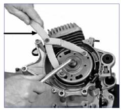
Remove the nut (right-hand thread).Fit the crankshaft end protector68007 onto the end of the crankshaft.
